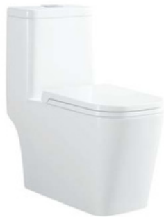
8803 Siphonic One-Piece Toilet Size: 685x370x780mm S-trap Roughing-in: 300-400mm
