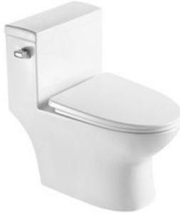
8974 Siphonic One-Piece Toilet Size: 690x410x700mm S-trap Roughing-in: 285mm
