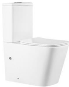
9901 Rimless Two Pieces Toilet Size: 630x340x850mm P-trap Roughing-in : 180mm S-trap Roughing-in: 100-250mm
