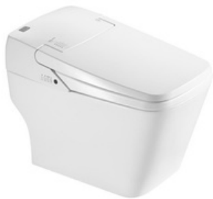
5002S Intelligent Toilet Size: 720x405x575mm S-trap Roughing-in: 300mm Hydraulic require: 0.3~0.8 Mpa
